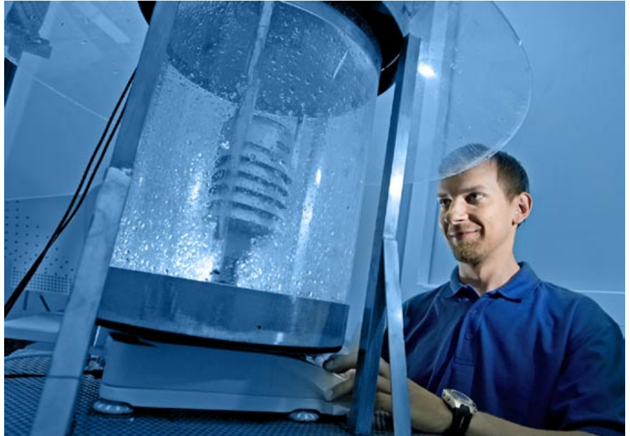
A WXT520 in the rain chamber in Vaisala.
